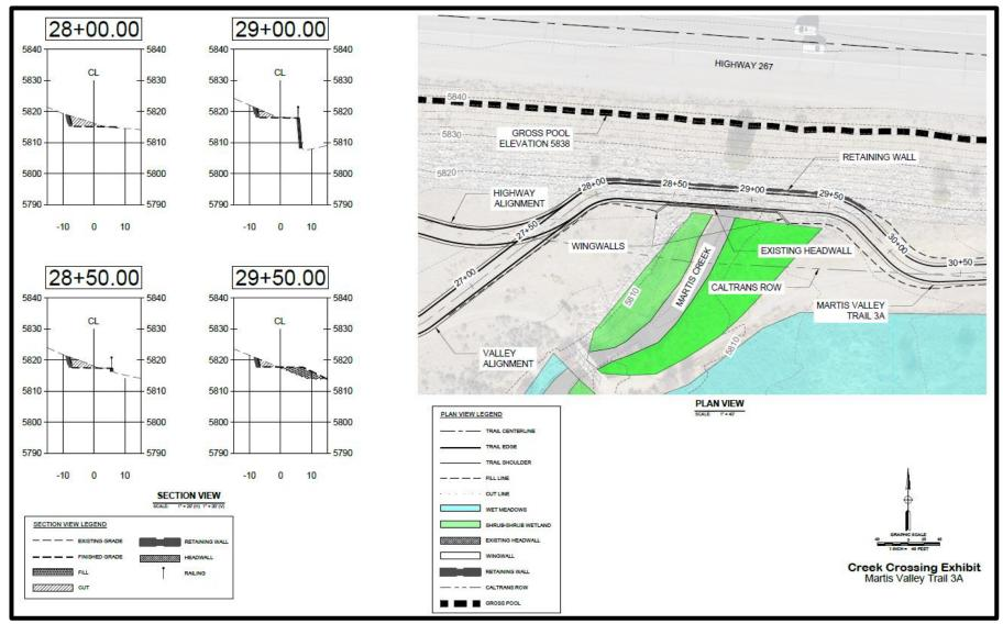
Figure 6. Proposed Creek Crossing Using the Existing Caltrans Culvert Structure.
